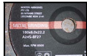
180mm DC Grinding Disc Denotes Maximum Operating RPM of 8500 ( Right wheel for this machine )
